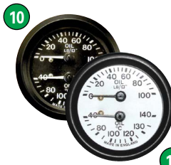
Oil Pressure/Oil Temp Gauge 0-100 PSI, 1/8" BSP inlet (oil line not included)/40-140°C, 7ft capillary, 3/8" BSP sender.
