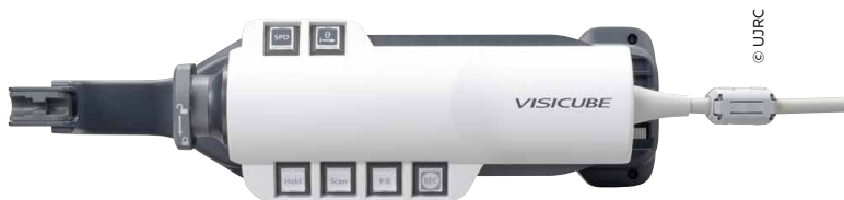
▲ Visicube's control unit with a miniaturised ultrasound device.
