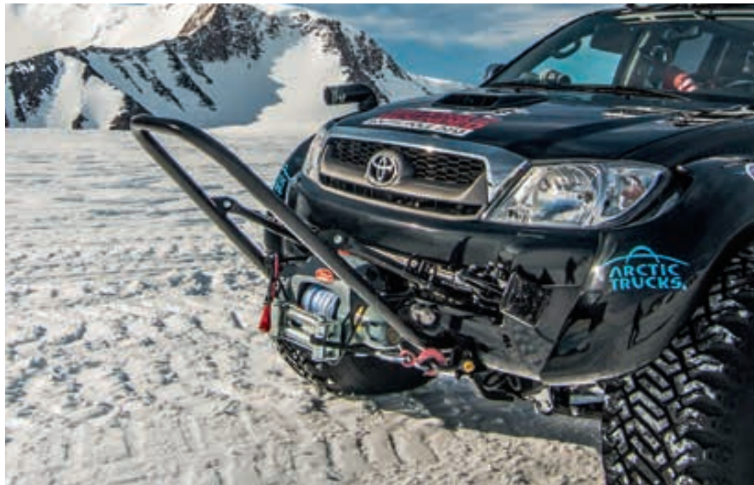
▲ Arctic Trucks rebuilds the vehicle frame, drivetrain and body, mounts special tyres, adds various specialized equipment and accessories and an electrical system to drive them.
