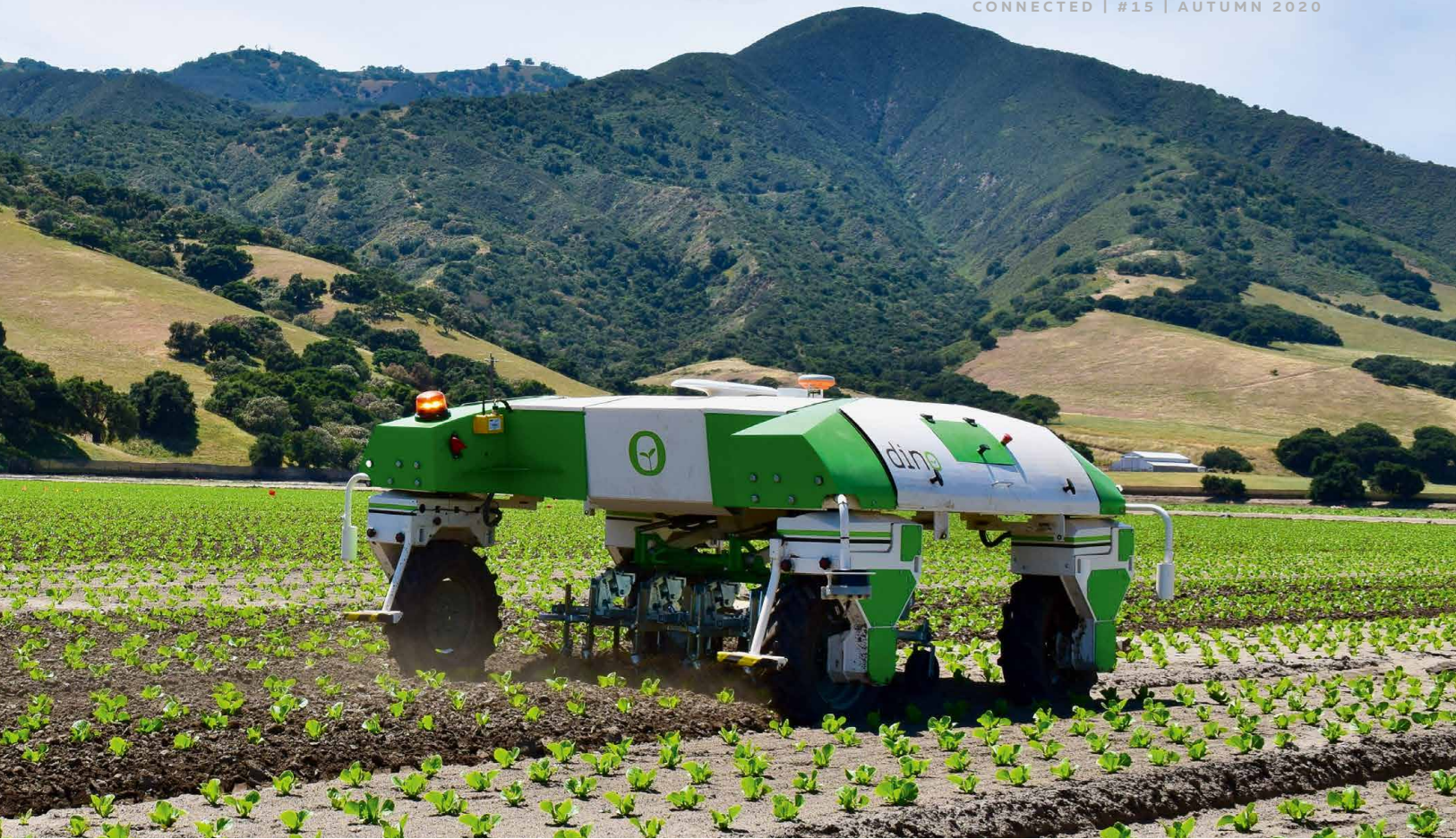
Two Dino robots in the fields. Each capable of weeding some thirty hectares autonomously.
