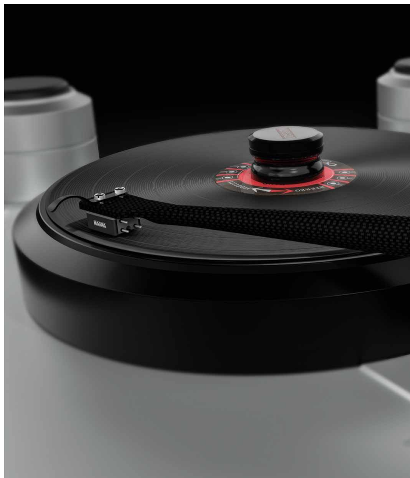
▲ To control parasitic vibrations, the carbon fibre tonearm wand includes a layer of wood with a silicone damping system.
