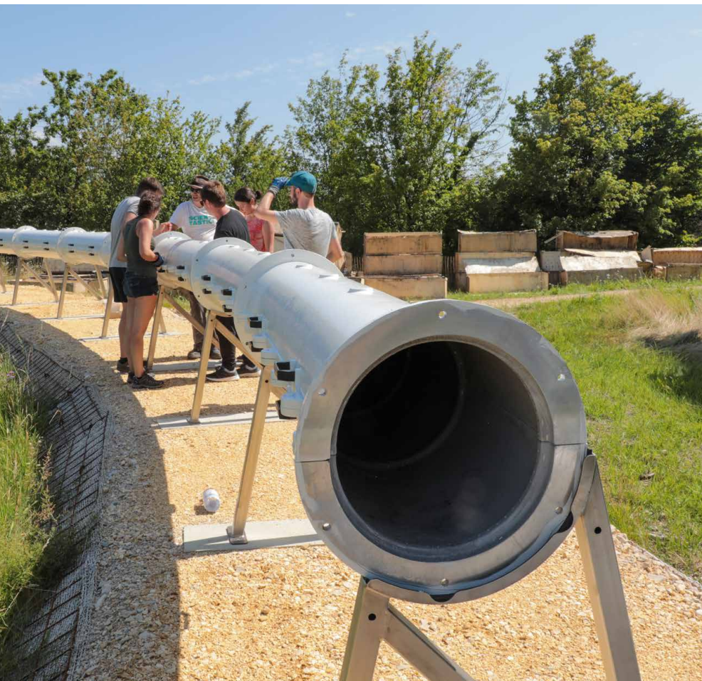
▲ Assembling the elements. Once completed, the test tube (designed on a 1:12 scale) measures 40 m in diameter.
