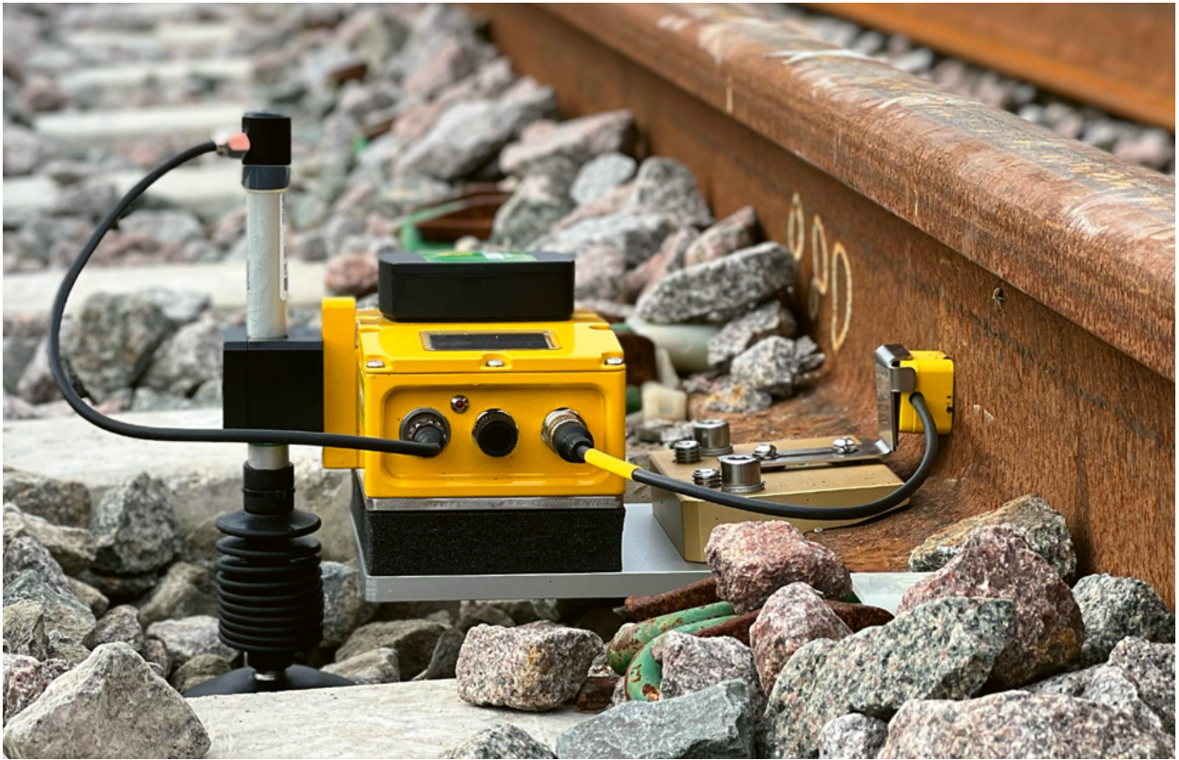
▲ RailSense: flexible, real-time monitoring for the assets that keep networks moving.
