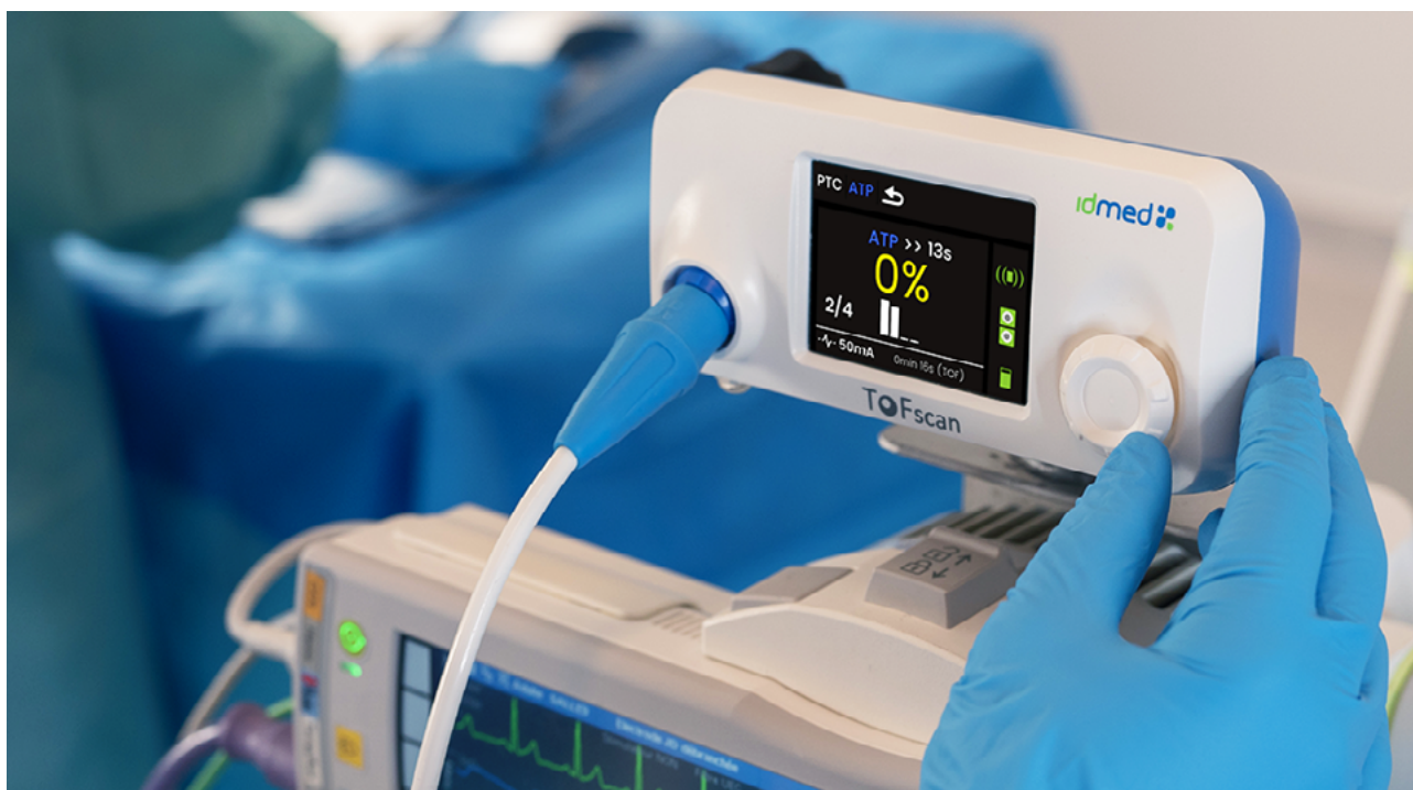
▲ TOFscan monitors neuromuscular blockade during anaesthesia.
