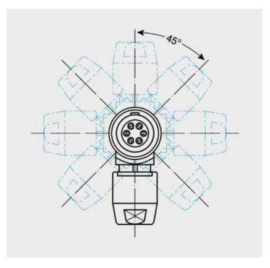
Right-angled connectors are well-known by users and are typically used for space-saving reasons or to avoid cable snagging issues. Upon customer request, LEMO has been adapting the cable outlet angle to either a 3, 6, 9 or 12 o'clock position by using specific components, according to the selected position. Anglissimo pushes the concept one step further.
