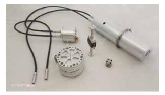
Top: Micromega actuators on the rear side of the telescope mirror (66 of these will be installed on the DAG telescope).
