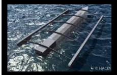
A French start-up HACE (Hydro Air Concept Experimental) has developed a machine that captures wave energy at very low cost and transforms it into electricity. The system uses simple floaters that, by rising and falling thanks to the waves, compress air in cylinders. Releasing this air activates a turbine that generates electricity. A first 200 kW industrial prototype should be ready by 2018 and this technology could provide up to 1 KW/m<sup>2</sup> with only 30-cm waves.
