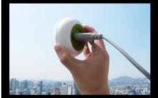
Two young South Korean designers have created an autonomous portable socket. The size of a big biscuit, Window Socket has a small solar panel on one side and a standard 2-pin socket on the other. It is enough to stick its suction cup on a window and solar energy is directly transformed into electricity! Then all you have to do is connect and charge, for example, your smartphone.
