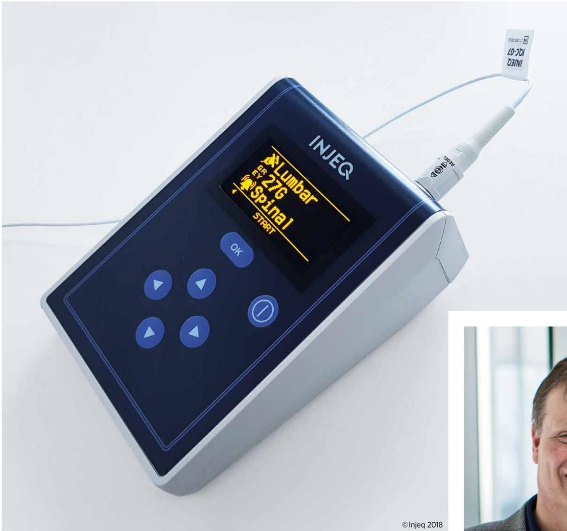
▲ The Injeq 301 tissue analyser identifies the tissue at the tip of the Injeq IQ-Tip needle in real time. The device is connected with a REDEL SP connector and a Northwire cable.
