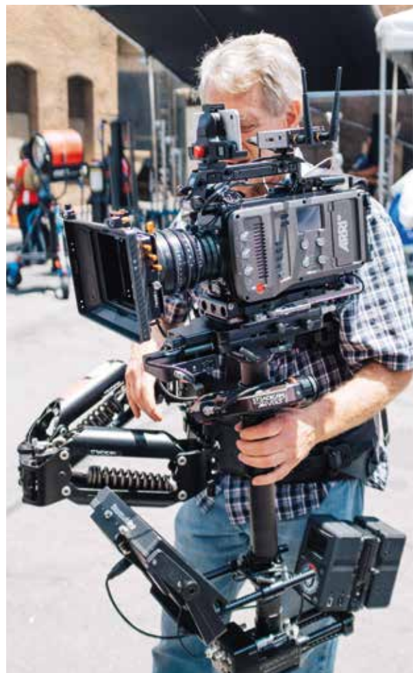
▲ The M-1 Steadicam is completed with an "exovest" and a lever-arm supporting the system, as well as a Volt System, a tool that provides operators with horizontal stabilisation.
