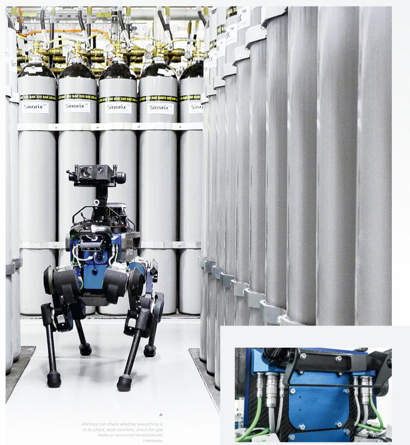
This quadruped robot was designed by ANYbotics, a spinoff of the Swiss Federal Institute of Technology in Zurich (ETH Zurich). Made of carbon fibre and aluminium, it weighs about thirty kilos. It is fully ruggedised, water- and dust-proof (IP-67). A kevlar belly protects its main body, carrying its powerful brain, batteries, network device, power management system and navigational systems.
