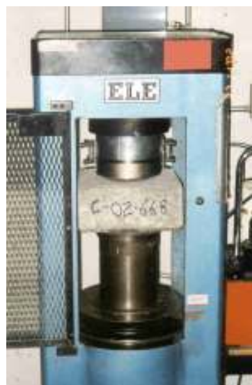
Figure 2 – Test set-up for simulated keyhole testing
