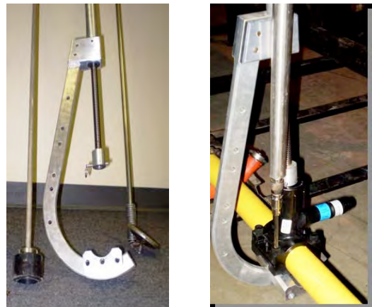
Figure 10: Keyhole tools used to clamp service tee in place. Courtesy Gas Technology Institute.
