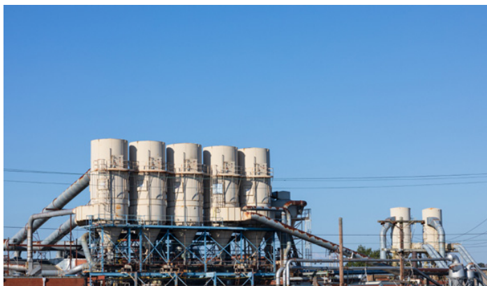
The efficiency of dust collector systems, like the ones found at this furniture plant, depends on the quality and performance of their pulse valves.
