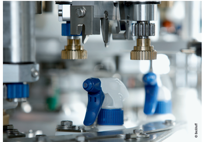
Weightpack also controls all secondary processes, such as capping the bottles, with PC-based control.
