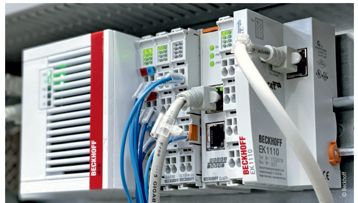
CX5130 Embedded PCs (shown here) or C6030 ultra-compact Industrial PCs are used depending on the system configuration.
