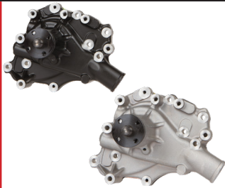
Standard rotation late water pump. 5-3/4" hub height, 5/8" shaft, 1-3/4" inlet. High flow. Available in cast or black.
