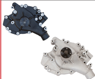
Big Block Ford standard rotation water pump. 5-1/2" hub height, 3/4" shaft, 2" inlet. High flow. Available in cast or black.
