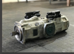
B30D & B40D Main Pumps exchange
