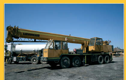
LIEBHERR 45TON CRANE
