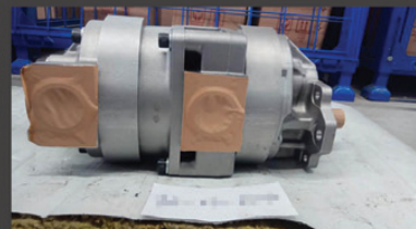
Komatsu WA600 pumps
