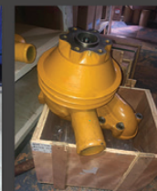
Komatsu 6D105 water pumps
