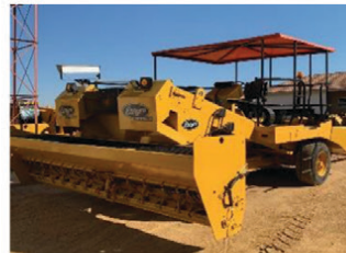
4 X Etnyre K Chip Spreader's Refurbished, mechanical and electronic operated
