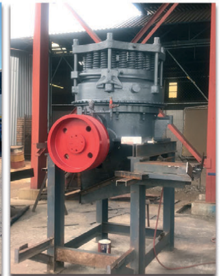
TELSMITH 5 X 24 CONE CRUSHER REBUILT WITH NEW LUBE SYSTEM & RECON MOTOR
