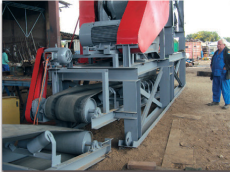
TELSMITH 14 X 24 JAW CRUSHER ON HEAVY DUTY SKID BASE WITH LOADING HOPPER AND VGF
