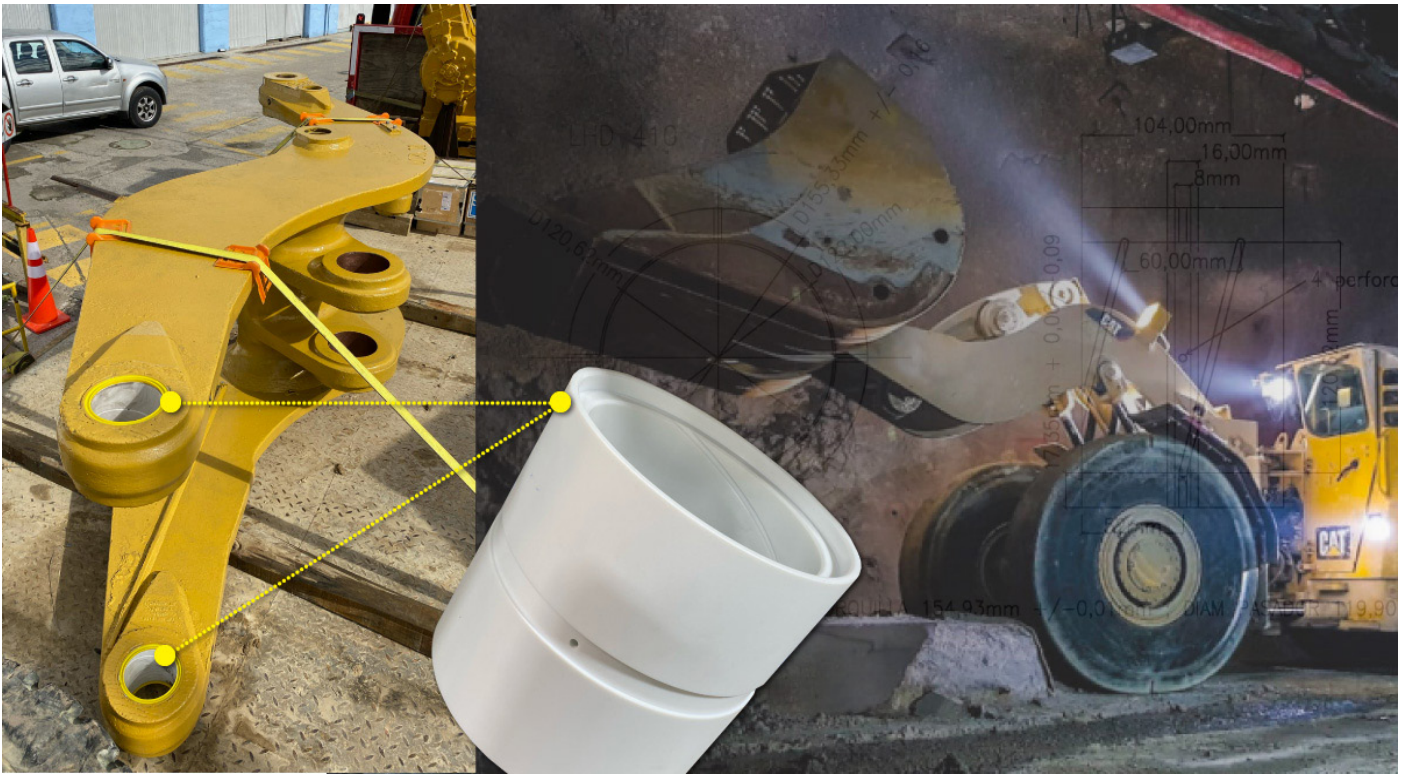
LHD booms fitted with Vesconite Hilube bushings
