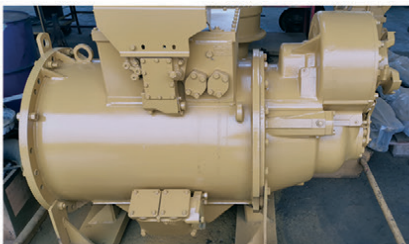
RECON 789C TRANSMISSION
