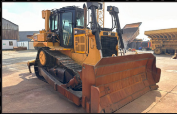
CAT D6R Track Dozer
