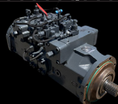
LIEBHERR R9350 Main Pumps
