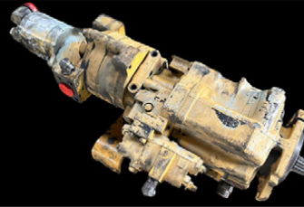
CAT 980H Main Hydraulic Pump
