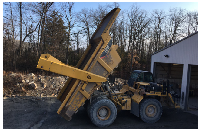
Operations can utilize Sideboards alone or pair them with Philippi-Hagenbuch Autogate® Tailgates to further increase capacity and prevent material from spilling from the back of the body.
