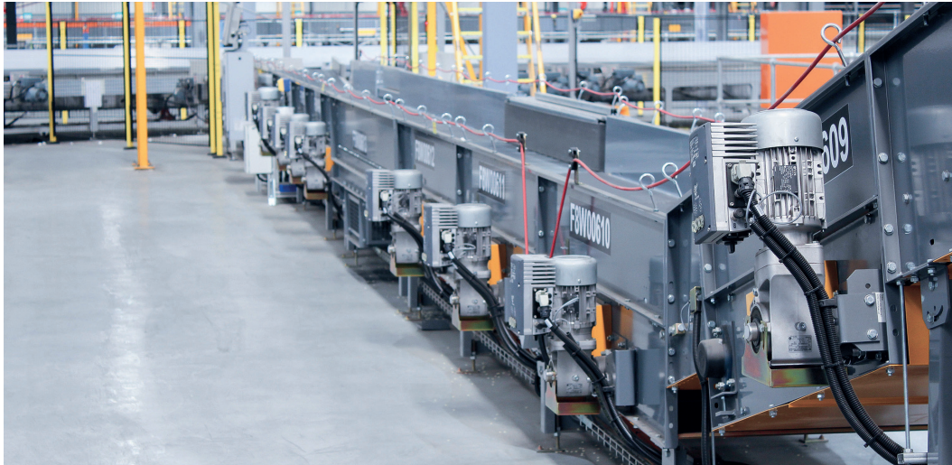
NORDAC FLEX SK 200E series frequency inverters have been especially developed for use in extensive conveyor technology systems.
