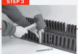
The two cemented surfaces must be stitched into close contact. Using a rubber mallet, pressure is best applied downward on a wooden block or blunt metal rod (not furnished). A firm surface under the belt in the area being stitched is required for best results.
