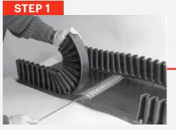
After stringing the belt on the system, insert the mechanical hinge pin in the fastener joint and clip the lock washers in place.
