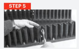
Complete the splice in the sidewall by inserting the flat head bolts through each end of the rubber corrugations. Place fender washers and lock nuts in place and tighten appropriately.
