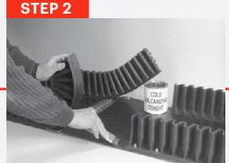
The loose ends of the sidewall and belt should be coated with two (2) coats of bonding adhesive. Using the special brush, work the cement onto both the bottom of the sidewall and the belt cover. Allow the first coat to dry completely; the second coat should be left tacky before sticking the two surfaces together. Holes punched at the factory should match up in their proper position.
