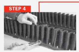
Once the stitching is complete, insert the flat head bolts from the bottom of the belt through the pre-punched holes (if applicable). Place the fender washer and lock nut in place and tighten appropriately.
