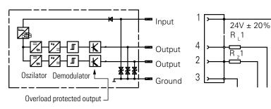
$R_1$ 1,  $R_1$ 2 = e.g. Coil Resistance of the switch relay >/ = 60 OHMS
