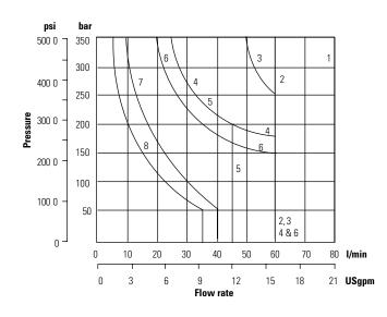
Graph 2 AC solenoid valves operating at 60 Hz
