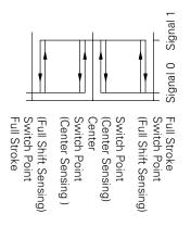
Signal 0 =Voltage at pin 2/4 < 1 .8V Signal 1 =Voltage at pin 2/4 > (Vs - 2.5V)
