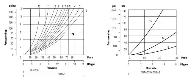
▼ Curve for spool type 6: not recommended for flows in excess of 60 I/min (15.8 USgpm).
