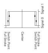
Signal 0 =V oltage at pin 2/4 < 1 .8V Signal 1 =V oltage at pin 2/4 > (Vs - 2.5V) Typical "PCD" output (For center se nsing 'a' port end, Full shift sensing 'b' port end)
