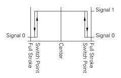
Signal 0 = Voltage at pin 2/4 < 1.8VSignal 1 = Voltage at pin 2/4 > (Vs - 2.5V)
