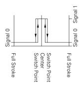
Signal 0 =V oltage at pin 2/4 < 1.8 V Signal 1 =V oltage at pin 2/4 > (Vs - 2.5V) Typic AL "PD A/P DB" output (For full shift sensing)
