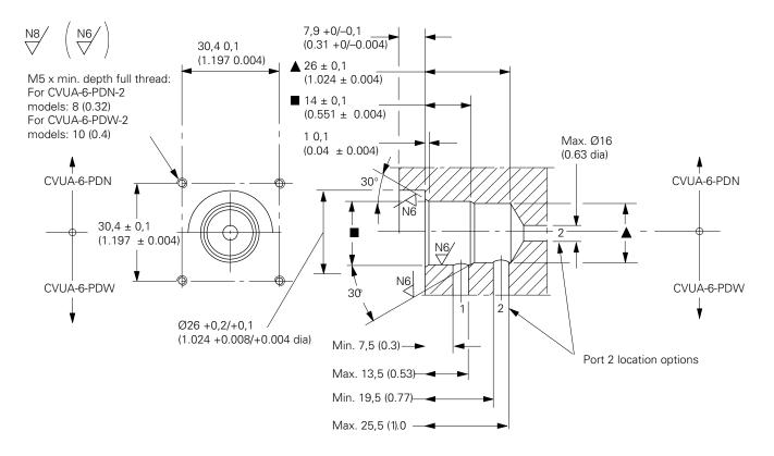
◆ Tool kit 638692 for machining the Ø18 mm and Ø19 mm bores (and when required, the Ø26 mm bore) can be ordered if required. The kit comprises a stepped drill and a stepped reamer.
