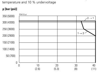
Measured with oil viscosity 33mm2/s (cSt), coil at steady-state
