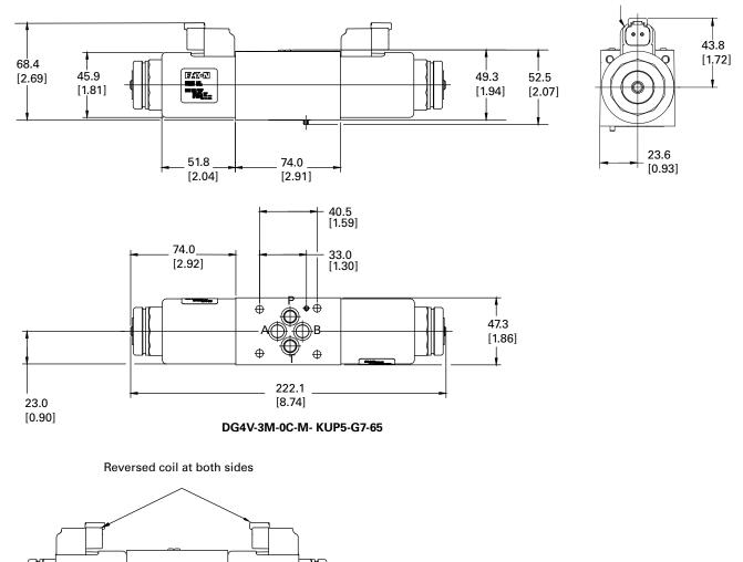
**Note:** Option RCA will have coil at A port reversed and option RCB will have coil at B port reversed.
