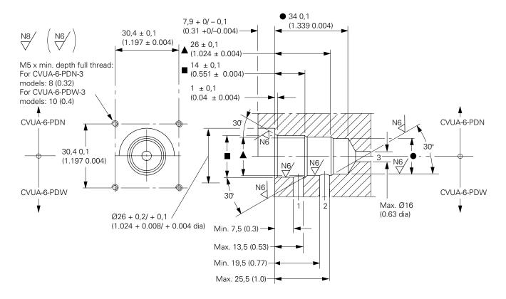
◆ Tool kit 459285 for machining the Ø17 mm, Ø18 mm and Ø19 mm bores (and when required, the Ø26 mm bore) can be ordered if required. The kit comprises a stepped drill and a stepped reamer.
