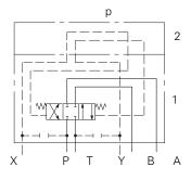
**Note:** That for clarity pilot lines (dotted lines in illustrations) are omitted from the main-stage nameplate.
