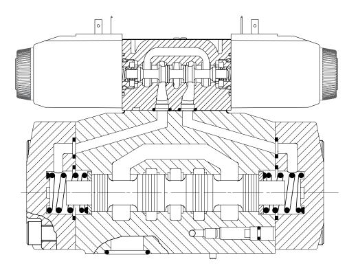
DG3V-7 30 Series, pilot operated directional valves
