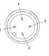
**Pin 1** is only used on the Z option for 24 VDC power to the valve.
