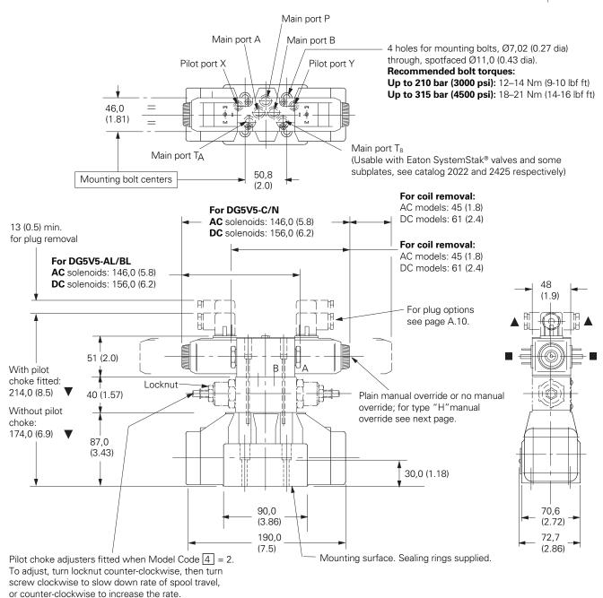
Re-tighten locknut to 25-30 Nm (18-22 lbf ft).
