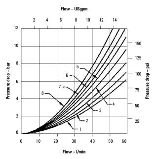
The pressure drop curves give approximate pressure drop  $\Delta P$  when passing 36 cSt (100 SUS) fluid(s) having a specific gravity. of .87.
