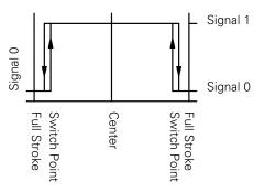
Signal 0 = Voltage at pin 2/4 < 1.8VSignal 1 = Voltage at pin 2/4 > (Vs - 2.5V)
