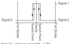
Signal 0 = Volt age at pin 2/4 < 1.8VSignal 1 = Volt age at pin 2/4 > (Vs - 2.5V)
