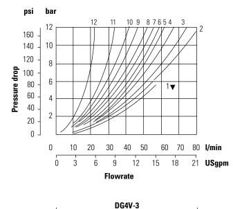
▼ Curve for spool type 6: not recommended for flows in excess of 60 I/min (15.8 USgpm).
