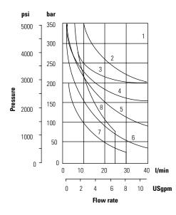
Typical with mineral oil at 36 cSt (168.6 SUS) and a specific gravity of 0.87.
