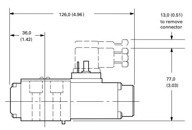
Dimensions are shown for standard connectors. For connectors with rectifiers and/ or LED this dimension varies up to 84,0 (3.31) maximum. Refer to double solenoid models below for port designations.
