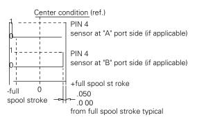
1 = voltage at pin 4 (Vs – 2.2V) min. 0 = voltage at pin 4 0.5V min.
