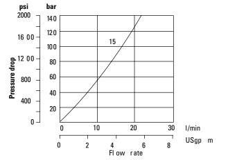
▼ Curve for spool type 6: not recommended for flows in excess of 60 I/min (15.8 USgpm).
