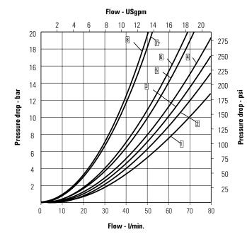
Typical with mineral oil at 36 cSt (168.6 SUS) and a specific gravity of 0.87.
