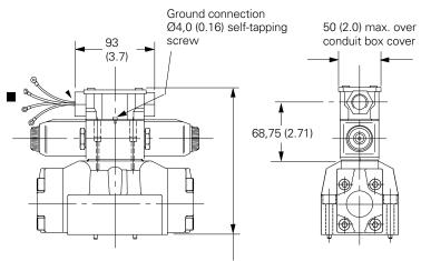
With pilot choke fitted: 227,0 (8.94) Without pilot choke: 187,0 (7.36)
