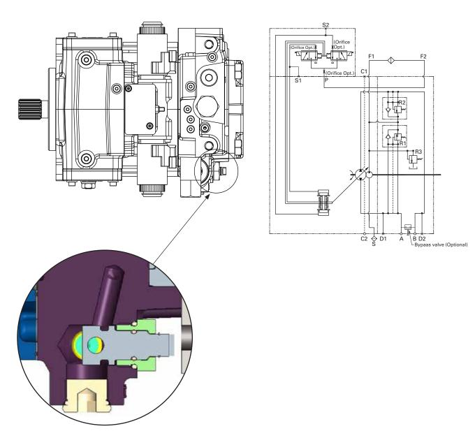
**Caution:** Towing for a prolonged time and distance may result in internal heat generation damaging the hydraulic system. Hence with appropriate safety accessories, check the oil level and bleed the air from the pump (If any) before restarting the pump.
