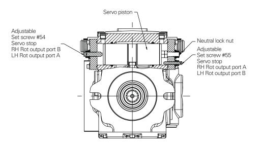
Internal pressure override control (IPOR) (Only available on X3 single pump)
