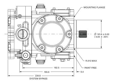
**Note:** The combined torque required for multiple pumps must not exceed the torque rating of the input drive shaft of the front piston pump. Consult an Eaton representative and/or Eaton engineering on side load recommendations.
