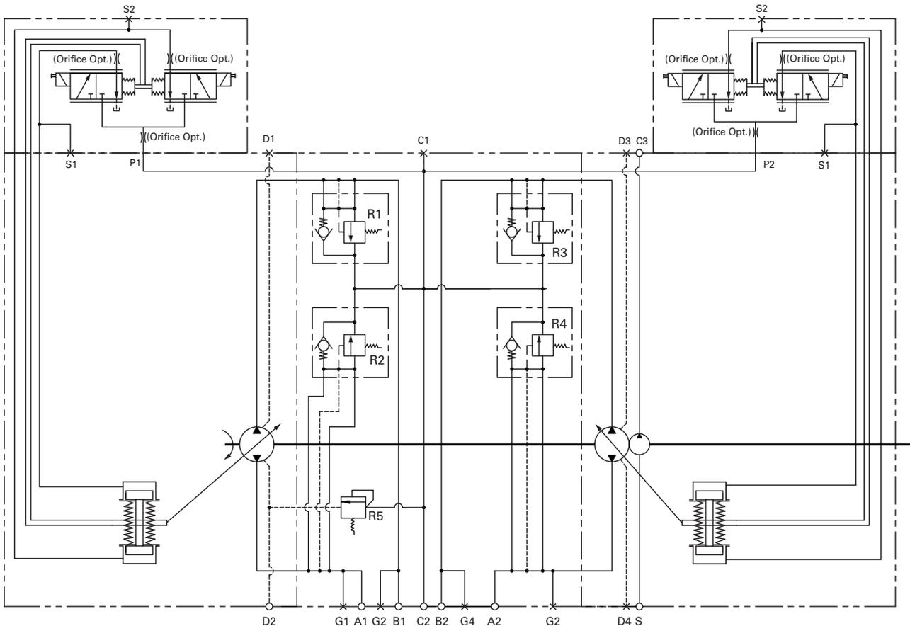
**Note:** An alternative braking system independent of the hydraulic brake should be provided to ensure the stoppage and holding of the vehicle in the event of hydrostatic power loss.
