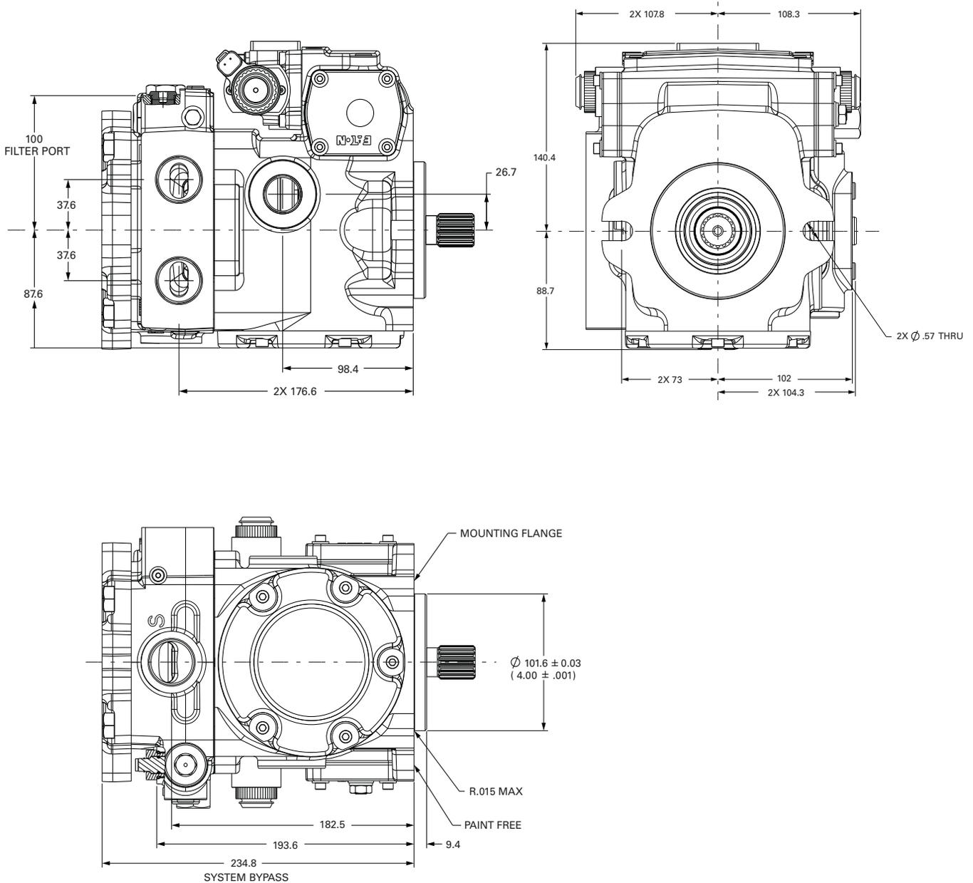
**Note:** The combined torque required for multiple pumps must not exceed the torque rating of the input drive shaft of the front piston pump. Consult an Eaton representative and/or Eaton engineering on side load recommendations.
