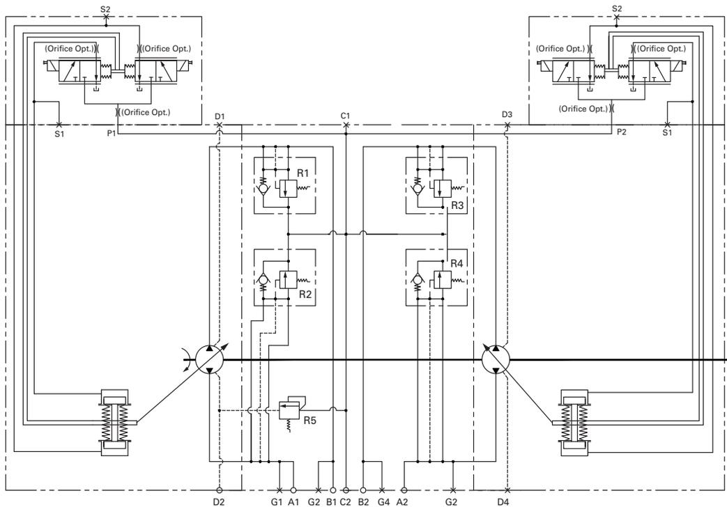
The Electronic displacement control (EDC) is ideal for applications requiring electronic pump displacement control. The EDC provides the flexibility of three command input choices. Control components include a proportional solenoid actuated valve assembly and an electronic solenoid driver module mounted on the pump.
