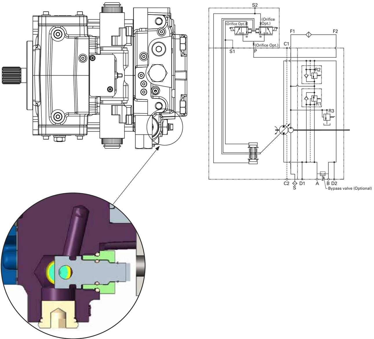
**Caution:** Towing for a prolonged time and distance may result in internal heat generation damaging the hydraulic system. Hence with appropriate safety accessories, check the oil level and bleed the air from the pump (if any) before restarting the pump.
