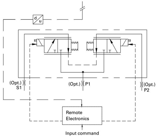
This control has an additional swash position sensor, which provides angular position of the swash plate very precisely at any point of time during pump operation. Swash position signal is converted in electrical signal and supplied to the Electronic Control Unit (ECU) of the hydraulic system. This signal is used to compare the input command to the pump and the output flow.
