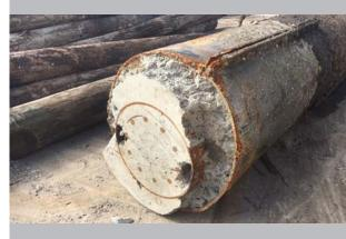
One of the steel and concrete piles.
