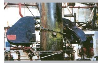
The band saw in position cutting 30" multistring casing
