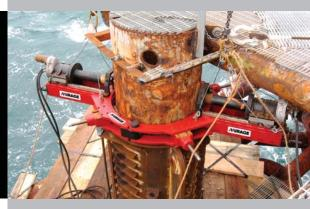
The DDU1636 machine in-situ drilling 6" pins.
