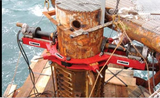
The DDU1636 machine in-situ drilling 6" pins.
