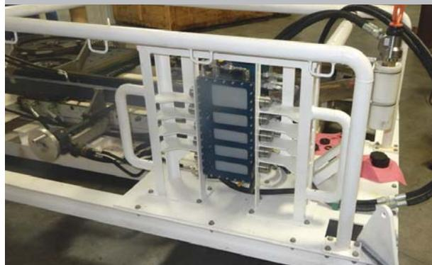
The manifold installed in the frame.
