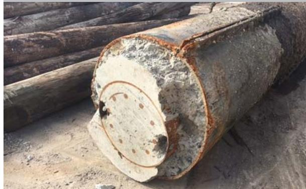
One of the steel and concrete piles.
