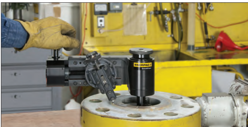
▼ The Enerpac FF-120 used to face a pipe flange.
