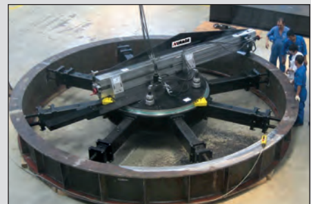
▲ Orbital milling machines used in shipbuilding and power generation industries.
