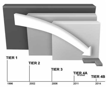
The Tier 4 Emissions Regulations established by the U.S. Environmental Protection Agency (EPA) and Canadian Environmental Protection Agency (CEPA) are getting tougher. In 1996, the first off-highway diesel emissions standard began with the implementation of Tier 1 regulations. Since then, standards have continued to be raised and will end with Tier 4B/Final in 2014.
