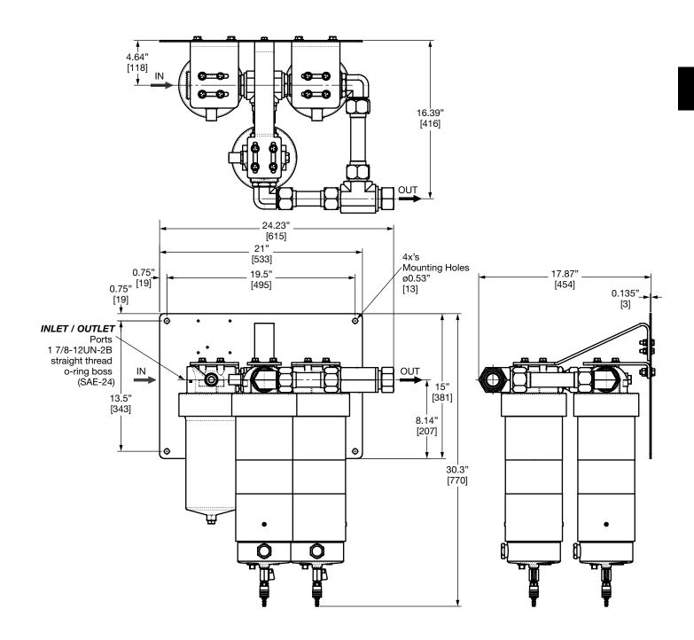
Dimensions shown are inches [millimeters] and for general information only. For complete dimensions please contact HYDAC to request a certified print.
