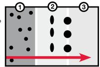
barrier sleeve traps droplets <25µ. This 3 elements in one prefilter, coalescing, and separation (most competitors have separate elements for each function) = smaller size! Tested per SAE J1488 (pressure side = smaller water droplets), with fuel down to 12 dynes/ cm IFT to replicate performance with more difficult fuels.
