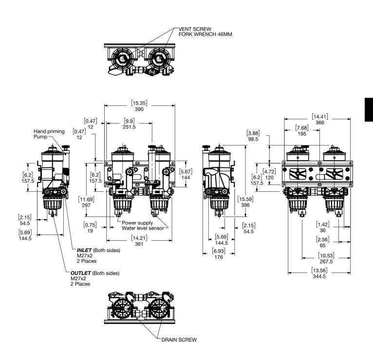
Dimensions shown are [inches] millimeters and for general information only. For complete dimensions please contact HYDAC to request a certified print.
