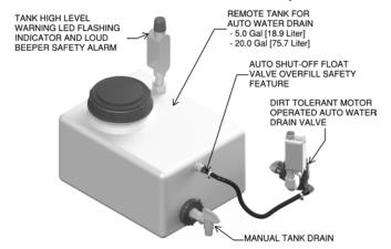
Note: Remote Tank dimension: 5 Gallon Tank: 22" W x 9.25" L x 7.125" H (558.80 W x 234.95 L x 180.97 H) 20 Gallon Tank: 15" W x 11" L x 31" H (381 W x 279.40 L x 787.40 H) Power supply for tank high level LED light: 9 VDC (battery included) Supplied w/ 9 VDC terminal for customer wiring provided.
