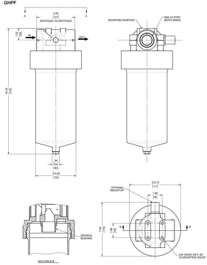
Dimensions shown are inches [millimeters] and for general information only. For complete dimensions please contact HYDAC to request a certified print.
