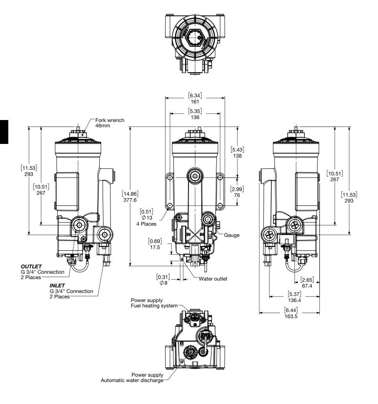
Dimensions shown are [inches] millimeters and for general information only. For complete dimensions please contact HYDAC to request a certified print.
