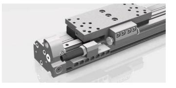
Oval piston provides an optimal distribution of transverse forces. Permanently connected to the slide, the oval piston can withstand higher loads and moments than the round piston. Users achieve the same performance with far more compact cylinders, which cuts down on weight and costs.
