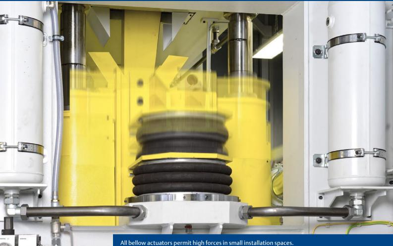
All bellow actuators permit high forces in small installation spaces. They operate practically without wear or the need for maintenance.
