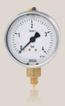
The model 113.53 Bourdon tube pressure gauge is produced with a stainless steel case. With its liquid filling it is suitable for use on measuring points with high dynamic pressure loads and strong vibrations.
