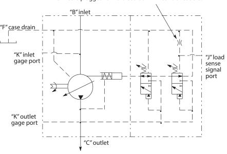
Optional bleed-down orifice in control Code B Orifice is plugged for no bleed down in control Code C.
