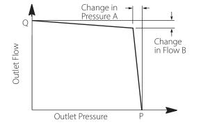
Pressure Cut-off Characteristics of Pressure Compensator Control @ 93°C (200°F), Static Conditions
