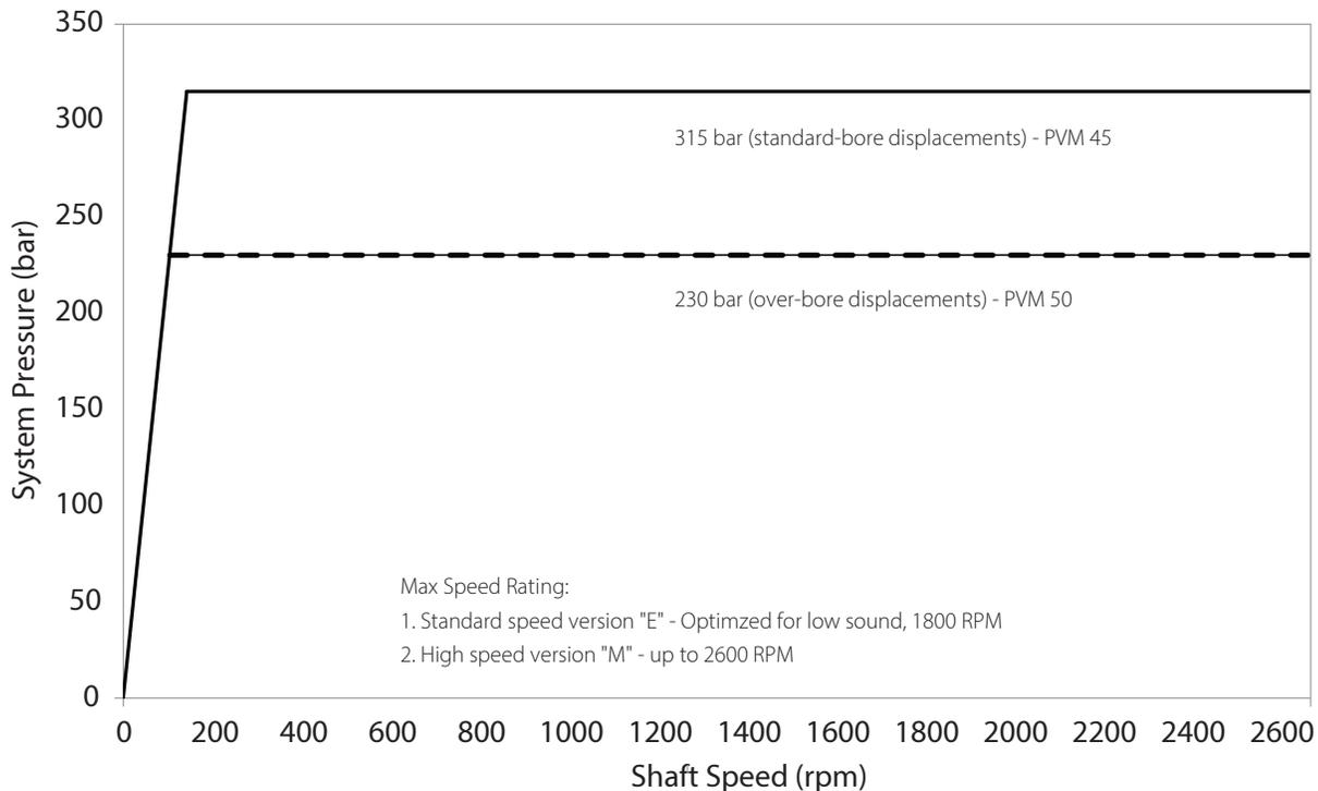
Test condition: Mineral oil SAE 10W, oil temperature 49° C (120° F), 1 bar absolute inlet pressure.
