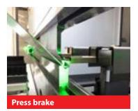
Highly accurate positioning, repeatability of machining cycles, and precise synchronization control of cylinders during the closing movement of the bending tool, are prerequisites of the hydraulic control system.
