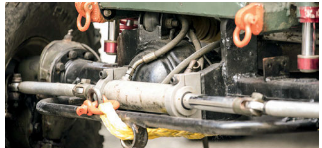
Full hydraulic steering and dual-caliper brakes are commonplace. The additional brake systems (one left and one right) are electronically actuated and linked to the turn signals; flip the signal and the vehicle cuts in that direction.
