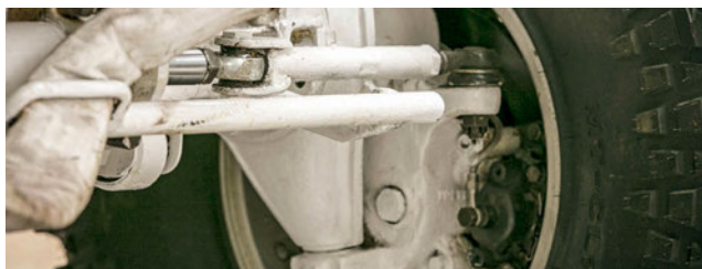
In deep mud, competitors running portal axles gain the advantage. The most commonly used is the Volvo 101 model.
