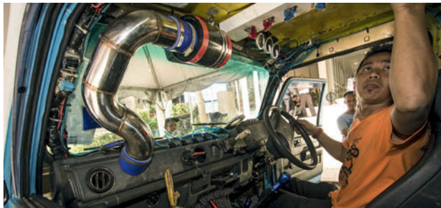
Hood-deep water is an everyday occurrence; air intakes are routed above the roof or inside the cockpit.
