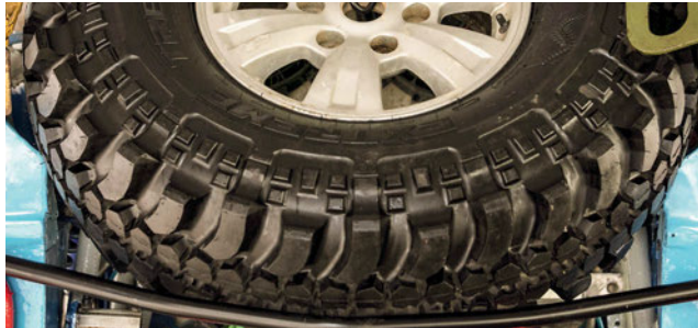
Extreme mud requires cavernous tread blocks and a means to extricate your vehicle. The most common choice of tyre is the Simex Centipede, Interco Super Swamper and Maxis Mud Trepedor.
