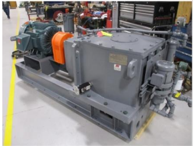
The repaired gearbox ready for shipment back to customer.
