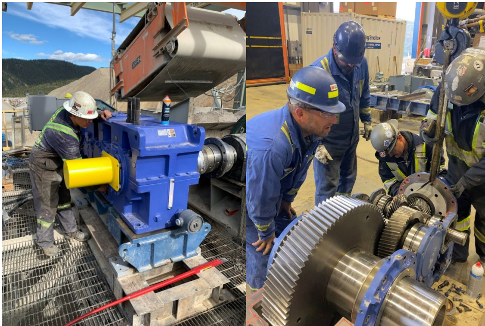
Figures 1 and 2: When a customer required gear reducer replacements, our team wondered if these failures could be the end result of a deeper equipment issue.
