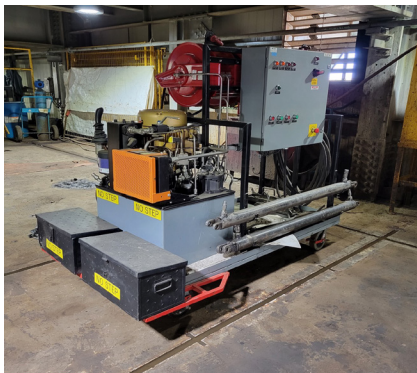
Figure 2: The new Motion design unit with integral hydraulic propulsion.
