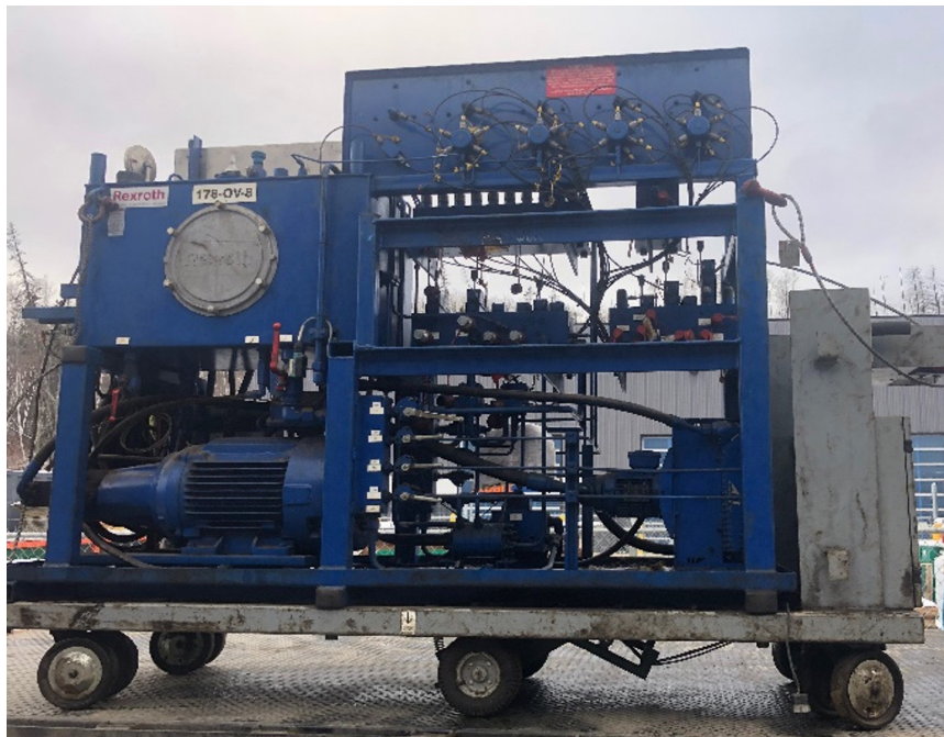
Figure 1: Original unit: The separate drivetrain suffered multiple failures, and the operation was not intuitive, described as "overly complicated" by the end user.
